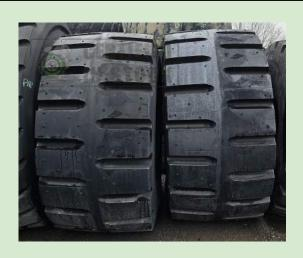
2pcs - 35/65R33 Polar Mold Retread Cut 601 L5 \*\* Repaired
